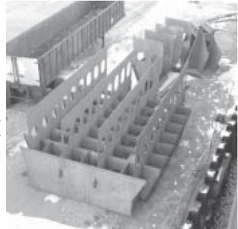
Right: Prefabricated main engine foundation.
